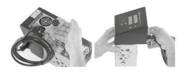
**ALWAYS** hold the SWID with one hand by the SWID attachment system (**CLAMP**) normally used to secure the SWID on a container. The other hand can be used as a guide by placing it on the metal structure on the front of the SWID.
